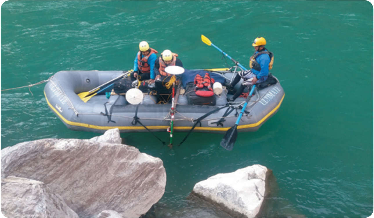
Bathymetric Survey Performed at Karnali River for Phukot Karnali Peaking RoR HEP
