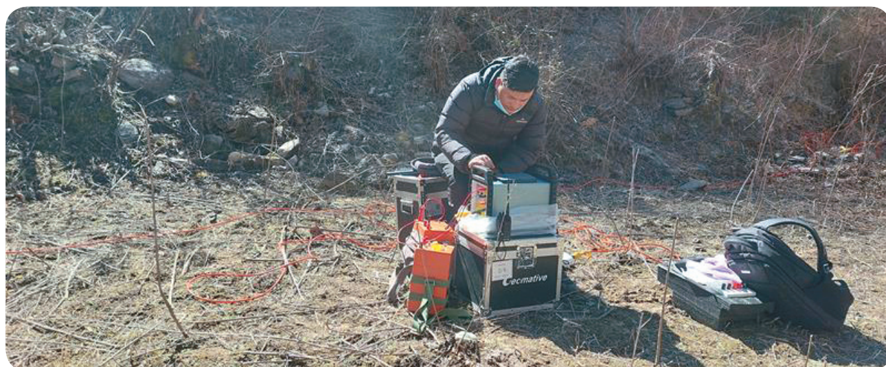
ERT Survey Works at JAHEP Headworks Area
